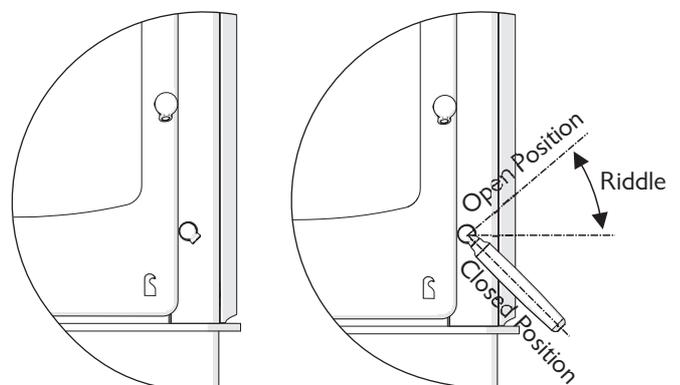
Door Opening Tool rotated 180° and pushed fully on to Riddler Knob
