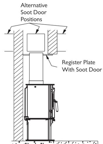
Fig. 9. Horizontal register plate with optional vertical rear flue connector
