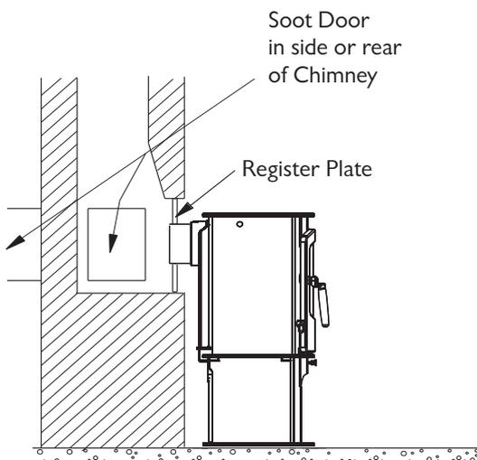
Fig. 7. Horizontal register plate with rear flue connection
